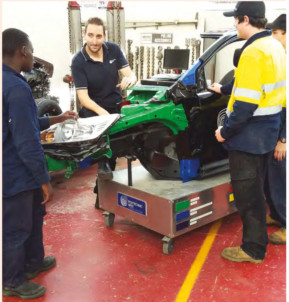
^ Lecturer Brendon Meinck shows a colour coded cut away vehicle to Certificate II in Auto Body Repair students. Brendon created the vehicle to show the different types of metals used in modern vehicles.
